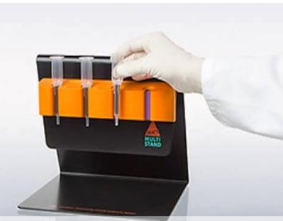
Magnetic bar (MACS separator) to hold the columns and attracted to the metal plate (shown black in colour above)
