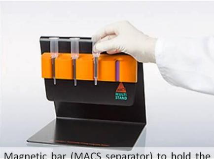
Magnetic bar (MACS separator) to hold the columns and attracted to the metal plate (shown black in colour above)
