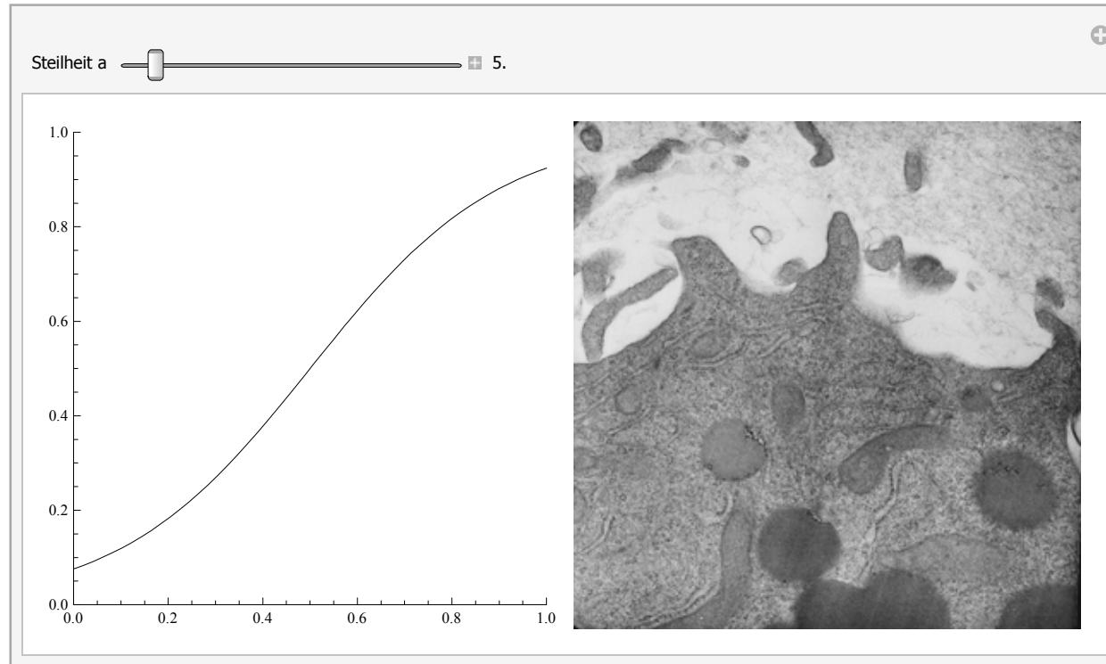
Tonwertkurve linear-potentiell (Variante 2):  $o = (c + 1) \left( (b + 1) i^\gamma - \frac{1}{2} \right) + \frac{1}{2}$
