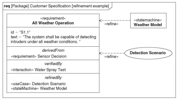
Note: This diagram demonstrates both Direct and Compartment Notation to represent a *refine* relationship. In practice, only one of these representations is needed.
